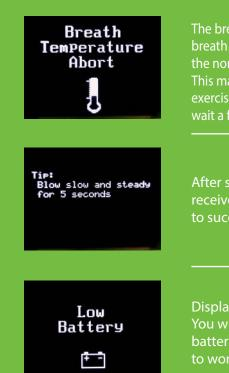
The breath temperature abort occurs when the breath blown into the device is inconsistent with the normal temperature of human breath. This may be due to you drinking an iced drink or exercising in the cold just before a test. If so, just wait a few minutes and try again.
